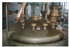
4991 Used 6000 Gal vertical 304L-SS Steel Tank. Internal rated 20 PSI @ 200 Deg F. Jacket rated 125 PSI @ 200 deg F. Dished Heads. 9' dia x 12' 9" T/T. (OAL: Approx 21'). Shell thickness: 3/8". 7.5 HP Lightnin Agitator, Model 93-C-7.5, 230/460V, 1725 RPM. Various top nozzles, 20" Top Manway, 20" Side Manway, 3" CBO. Built by Brighton Corp, 1986. S/N: ER-3030-3, ASME
